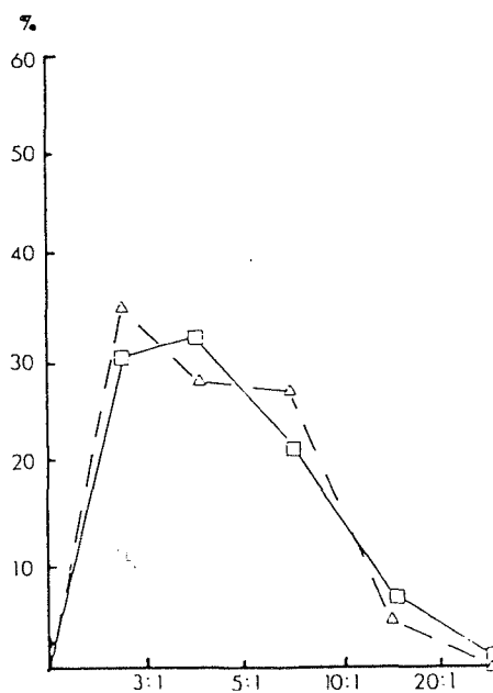
FIGURE 8. Percent amphiboles in each aspect group for a sample handled in two ways: solid line shows results using traditional method and dashed line shows results using centrifuge method. Dimensions of 100 particles measured for each curve.
